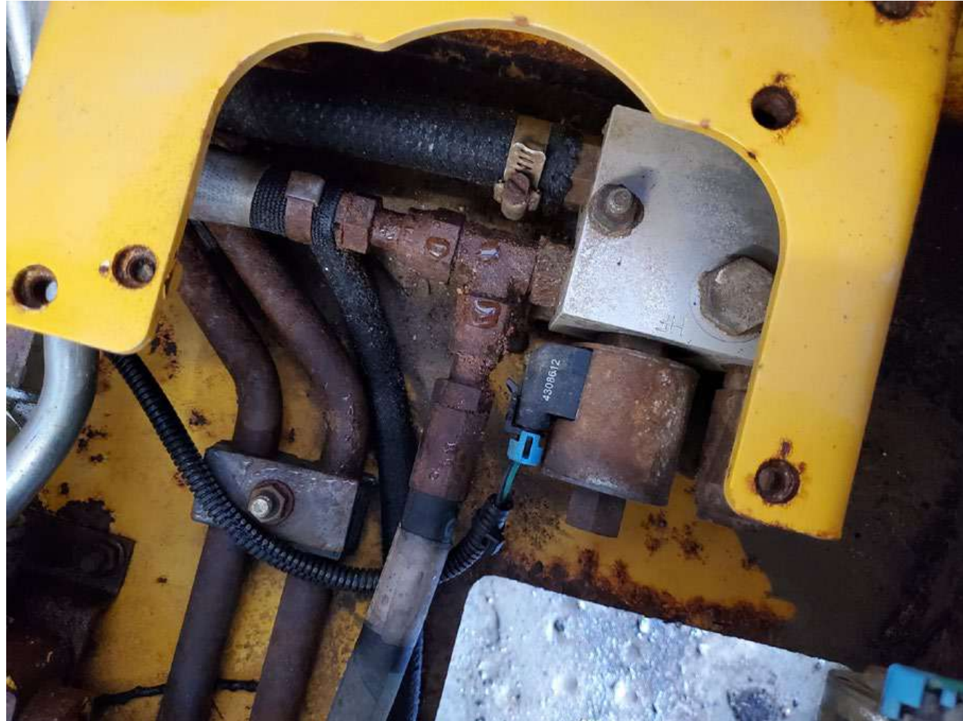
C:\Users\ccosgrove\Documents\2022 Budget pictures\323 Mini track Loader\Hydraulic steel lines corrosion.jpg
