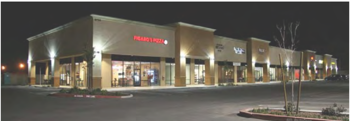
Provide adequate illumination that is continuous across the building facade. Views between interior and exterior through the location of windows.
