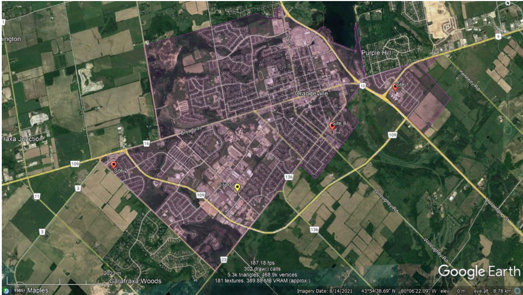
Figure 22 – ROM Coverage Design Map – Red Circles represent 39 optimal locations for a baseline VHF Conventional site constellation and PSBN RF equipment co-located at those sites. Cyan circles represent “fill-in” coverage sites for just 700MHz PSBN spectrum. Site 2 and Site 8 are proposed in the design (see full report for details).
